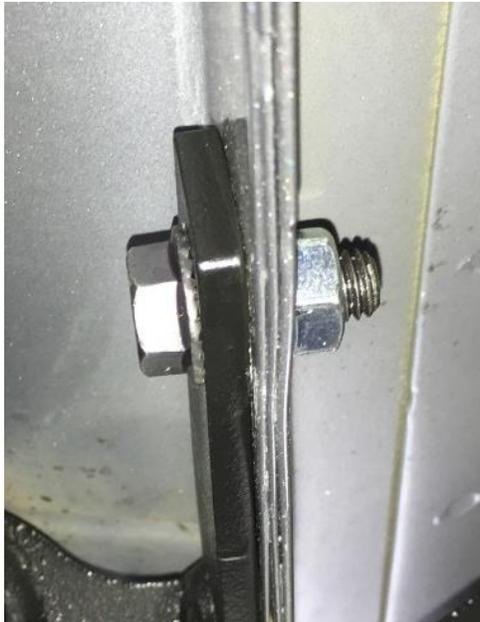
**Step. 6:** After final positioning, completely tighten all (x4) ¼"-20 x ¾" in the pinch weld attachment.
